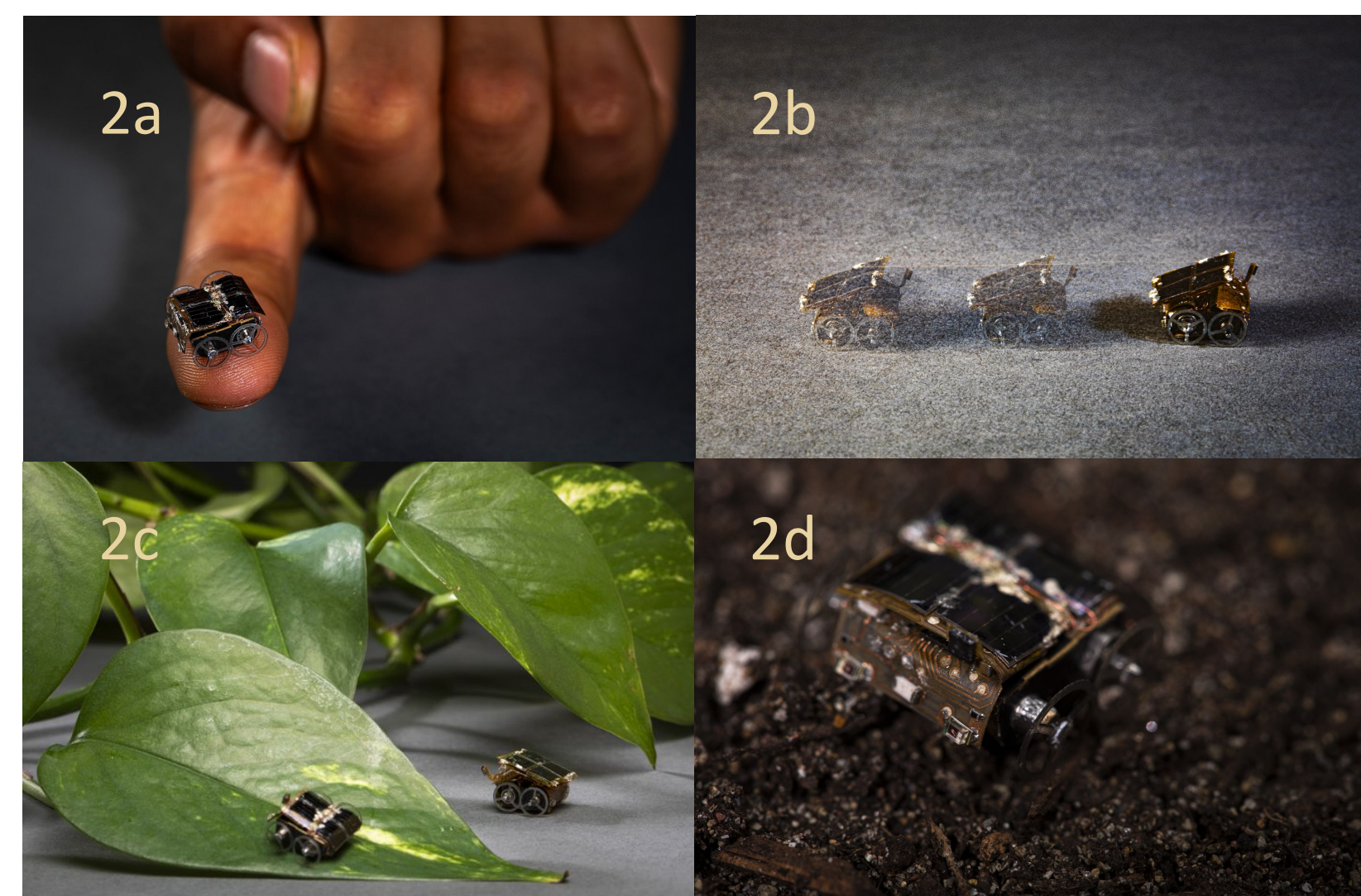
Fig. 2a) MilliMobile on the tip of a finger Fig. 2b) MilliMobile moving across a flat plane Fig. 2c) MilliMobile moving across a leaf Fig. 2d) MilliMobile moving across soil
